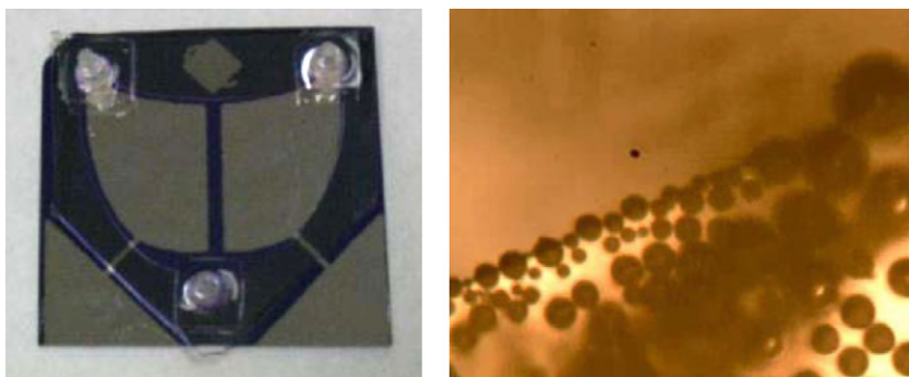
Fig. 3. Photo of a planar electrolyzer and a microscope image of bubbles generated on top of a Pt electrode. Note that there is no bubble formed on top of bared oxide.
